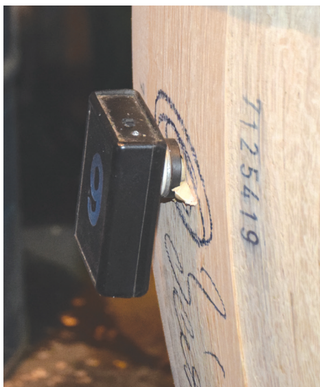
A heat sensor measures temperature inside the staves during the toasting process.
